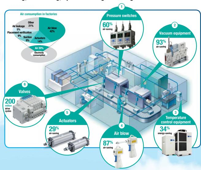
**Achieving Lower CO<sub>2</sub> Emissions During Manufacturing Through Space-Savings And Component Reductions.**
