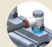
Leaks from pipe connections due to installation errors
